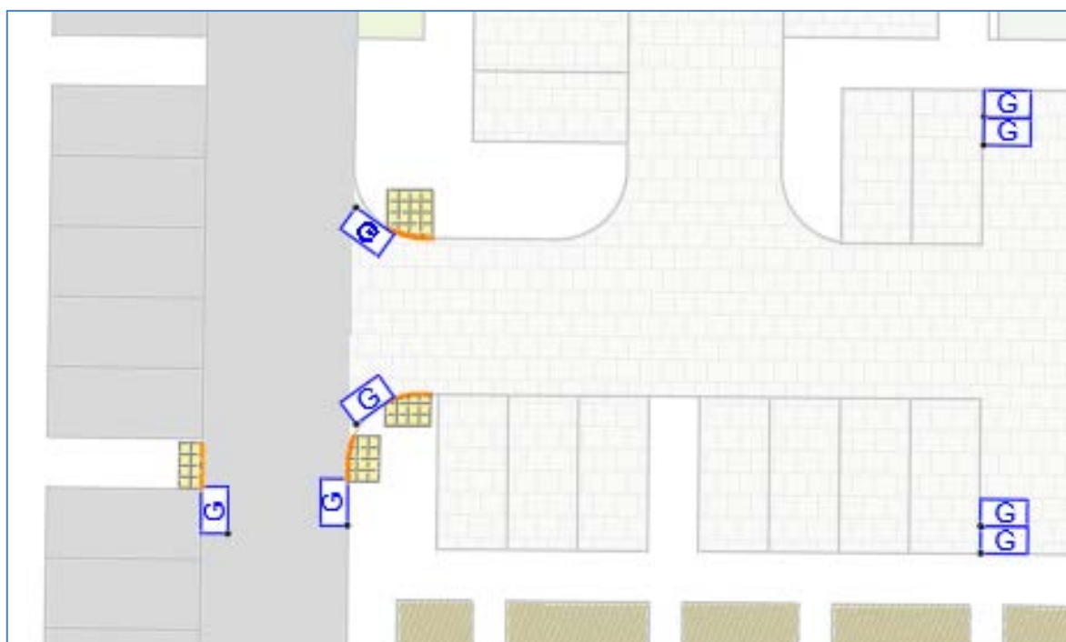
Figure 13 - Example of pedestrian crossing and shared surfaces
