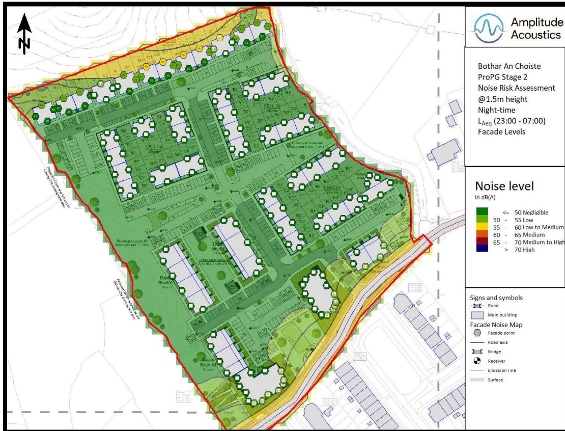
Figure 8: Predicted L_{Aeq,8hr} noise levels across the proposed development site including the acoustic screening effect due to the proposed buildings and boundary walls.
