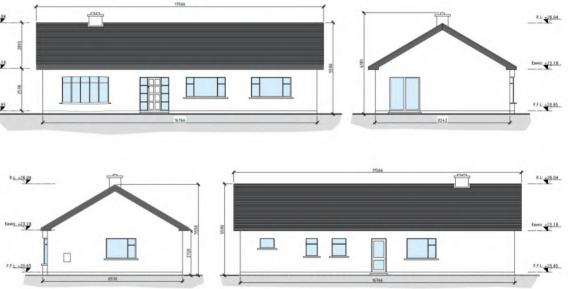
Figure 15. Extract from survey drawings showing the existing habitable bungalow situated to the South west of the site to be demolished
